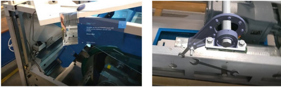
Fig. 3.11 Impression of MS Guides virtual display (left) and REFLEKT One 3D animation (right) in the MS HoloLens 2 application
