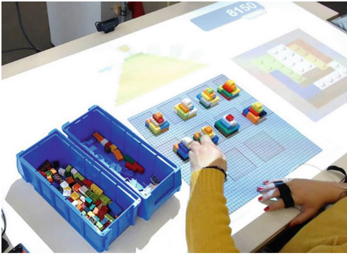
Fig. 10.5 Setup for an emotion-aware assistive system in production, using pyramids in various colors with identical geometry to simulate redundant work tasks
