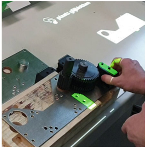
Fig. 3.15 Application of projection-based technology in manual gear box assembly in Company H
