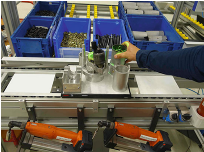
Fig. 10.10 Projecting information and feedback right into the workspace and even directly on a user's hand reduces the distraction from the work task
