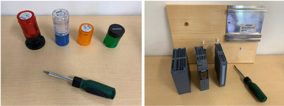
Fig. 8.4 The signaling column ( left ) and PLC task ( right ) that were used to evaluate Lenssembly. Both assembly tasks require a screwdriver
