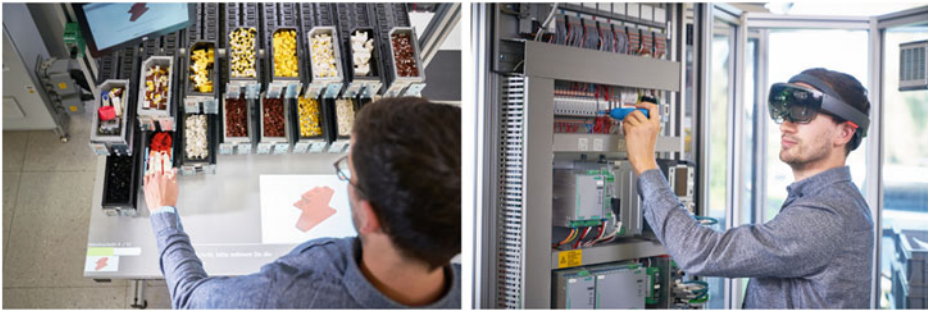
Fig. 4.1 Examples for industrial assistance systems based on in-situ projections (left side) and a head-mounted display (right side)
