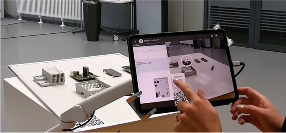
Fig. 6.4 An assembly use-case, with relevant information placed on top of their real-life counterparts via AR
