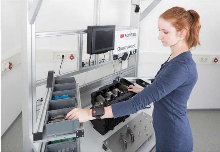
Fig. 10.2 The system “QualityAssist” by Sarissa was based on ultrasonic waves. It was one of the first systems allowing continuous process tracking
