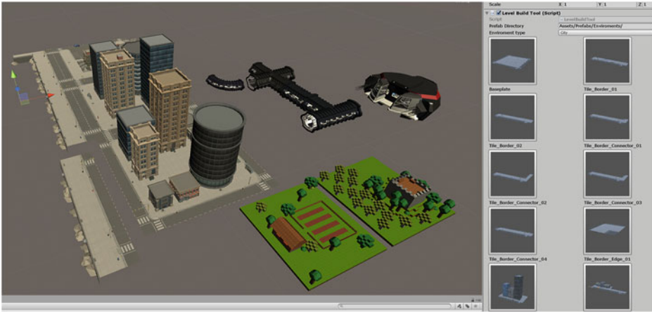
Fig. 7.7 Example test environment building blocks: Navigation guidance testbed creation using our customized Unity editor interface
