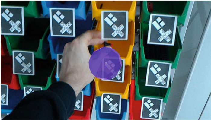
Fig. 7.6 Example use of the larger picking test environment “set” in a guidance test
