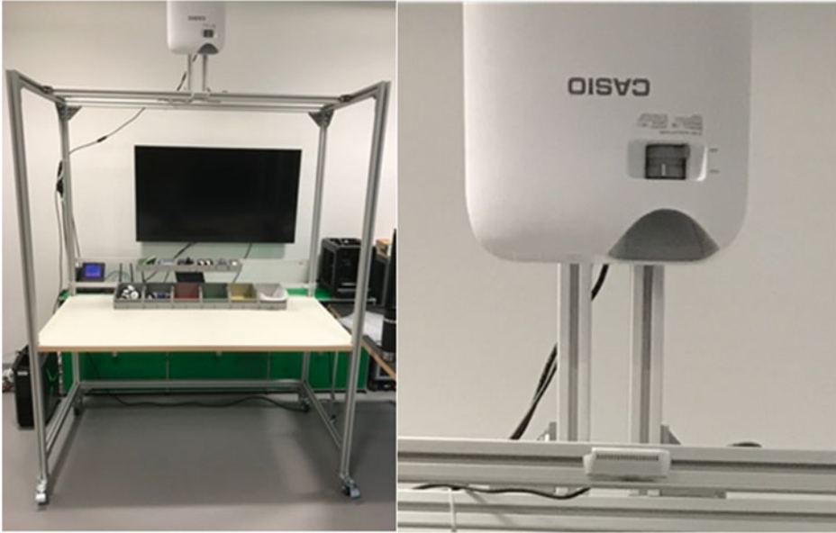
Fig. 5.2 The workbench mockup used as a base for the assistance system (left) and a close up of the camera at the bottom and projector at the top (right)
