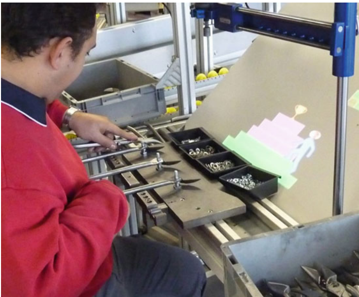
Fig. 10.8 A worker assembling metal shears. The pyramid gamification is projected directly in front of the workspace
